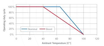
Values obtained with the motor screwed on an aluminum plate (dimensions 150 x 150 x 6 mm)
