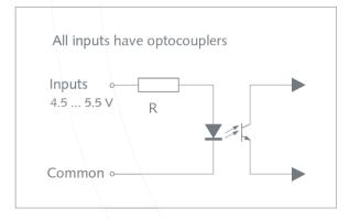
R = 470  $\Omega$ , excepted for the pulse input R = 220  $\Omega$ .
